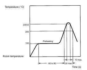
**Note:** The above curve is given on condition that the thickness of the PCB is 1.6 mm.
